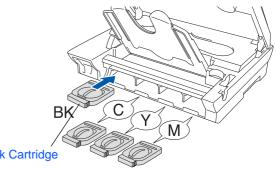
6 Close the ink cartridge cover, the output paper support and the scanner cover. When the DCP is setup for the first time, the machine will prepare the Brother unique ink tube system for use for the first time. This process will occur only once, the first time ink cartridges are installed. The preparation process will last up to four minutes.
